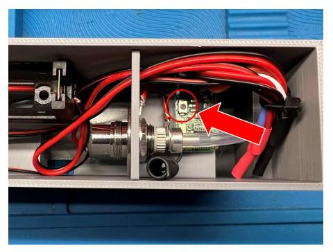
To program the remote press this button 1 time and wait for the blue light to come on. Now press the yellow button on the pedal remote and you will see the blue light blink. This means it is programmed. Test it by clicking the yellow button a couple of times and the fogger should turn on and off.
