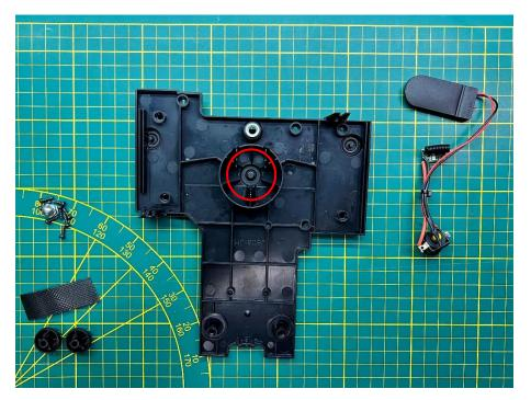
Once this is in place remove the double sided tape from the remote and from the battery holder and tape them as per picture below on the bottom plate.
