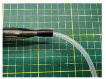
If needed some tape or heat shrink can be used to secure the hose.
