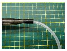
If needed some tape or heat shrink can be used to secure the hose.
