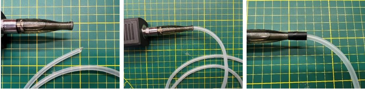
If needed some tape or heat shrink can be used to secure the hose.
