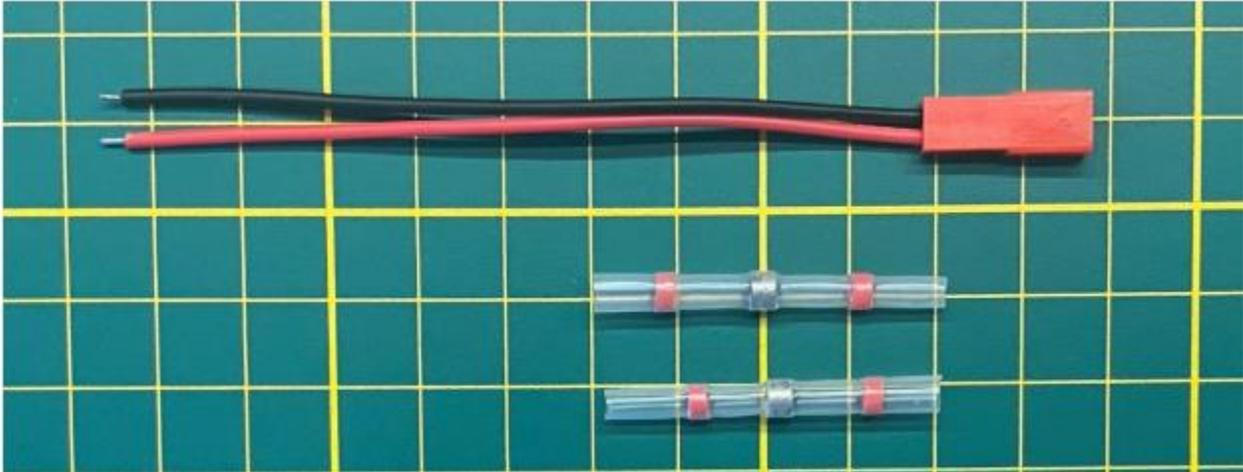
The soldering tubes can be used to attach a (wired) LED or any other 3.5 - 5v device to your smoke machine. If connected to the machine this will automatically turn on and off with the smoke machine using the remote. Simply slide one tube over each of the black and red wire and attach the led or device to the black and red wire. Now heat up the tubes with a lighter or a fan after which you will see the tube shrink to the wire and silver solder melting the 2 wires together.
