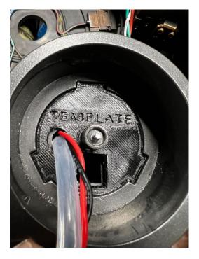
The template print will help identify the correct placement for holes which will allow the silicone tubing and LED power wires to pass through, as well as the port opening for the blower fan. Place this with the word TEMPLATE facing up for the proper orientation.
