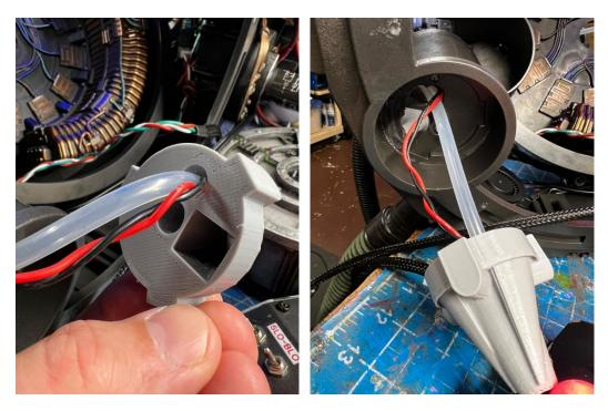
The LED and wires should be installed first, pushing the LED to the very tip of the cone. Once in place, the silicone tubing can be inserted 2-3cm (1/2") into the same hole to keep the wires (and LED) in place. Adding some hot glue will keep these in place and prevent smoke from escaping out this hole in the cone. Once those are installed the tubing and wires can be gently pulled through the drilled hole as the cone is pushed into place and secured using the original screw.
