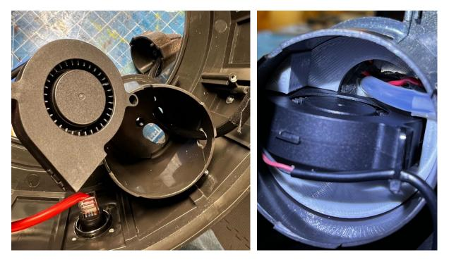
Once the holes are drilled you can simply insert the blower mount into the socket from below. There will be space to access the screw which holds the cone in place, as well as routing the silicone tubing and LED power wires. The blower will be held in place by the other half of the inner cyclotron housing once reassembled--this should be done last, after the cone has been fully installed and tested.
